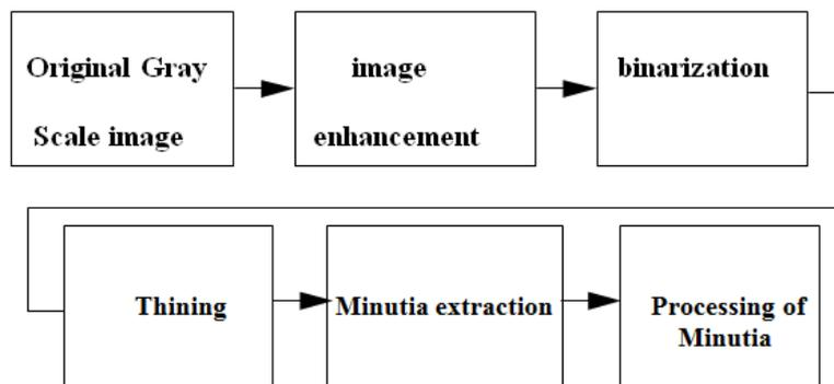
Figure 2. Process of Minutia Calculation
