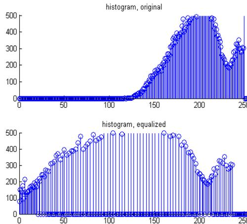
Figure 6. Histogram before and after Histogram Equalized
