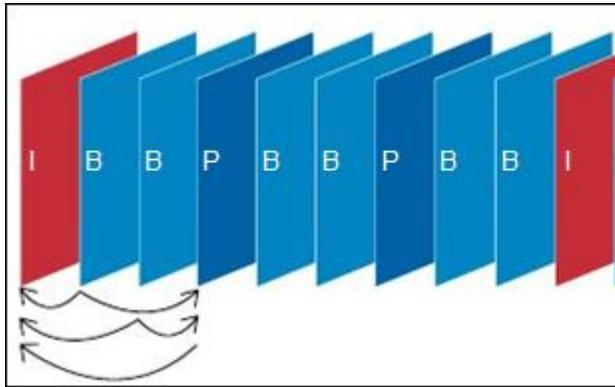
A typical sequence with I-, B- and P-frames. A P-frame may only reference preceding I- or P-frames, while a B-frame may reference both preceding and succeeding I- or P-frames.
