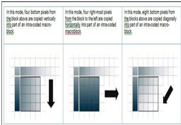
Illustrations of some of the modes that intra prediction can take in coding 4x4 pixels within one of the 16 blocks that make up a macroblock. Each of the 16 blocks in a macroblock may be coded using different modes.
