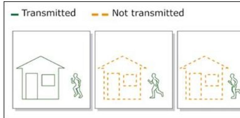
With difference coding (used in most video compression standards including H.264), only the first image (I-frame) is coded in its entirety. In the two following images (P-frames), references are made to the first picture for the static elements, i.e. the house, and only the moving parts, i.e. the running man, is coded using motion vectors, thus reducing the amount of information that is sent and stored.
