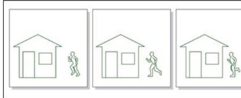
With Motion JPEG format, the three images in the above sequence are coded and sent as separate unique images (I-frames) with no dependencies on each other.
