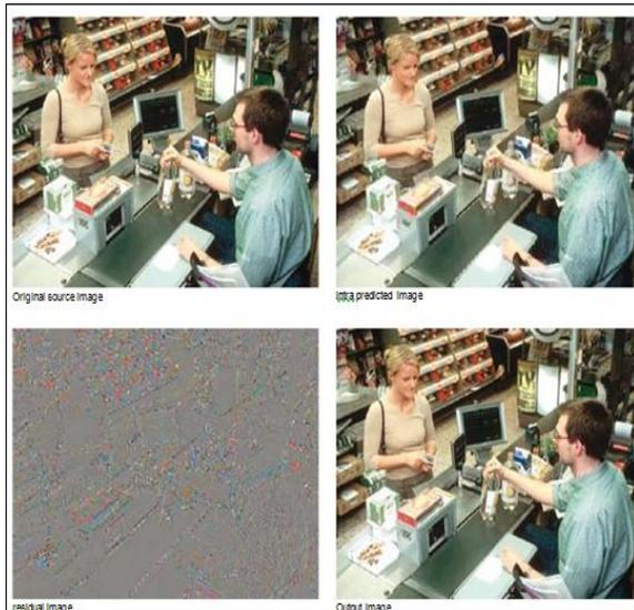
The above images illustrate the efficiency of H.264's intra prediction scheme, whereby the intra predicted image is sent for "free". Only the residual content and the intra prediction modes need to be coded to
