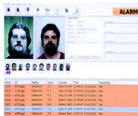
Fig(3) Face software compares the face print with other images in the database.
