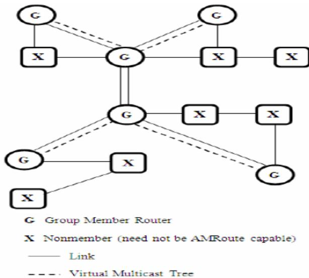
Figure 6: Virtual multicast tree formed by AMRoute
