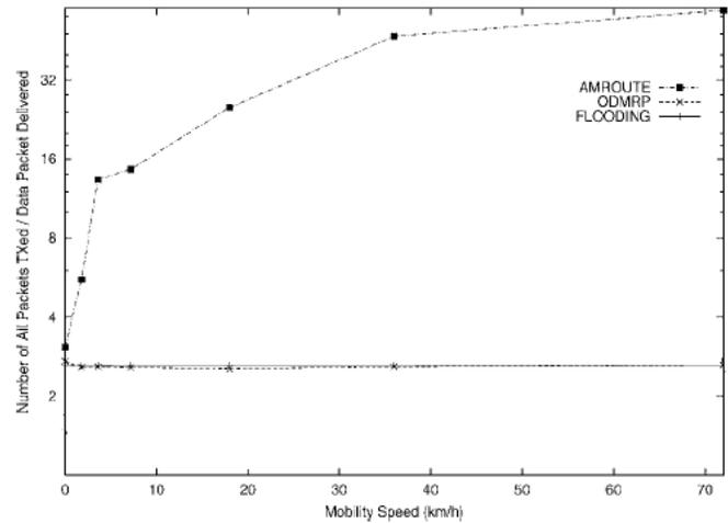
Figure 10: Number of total packets transmitted per data packet delivered as a function of mobility speed
