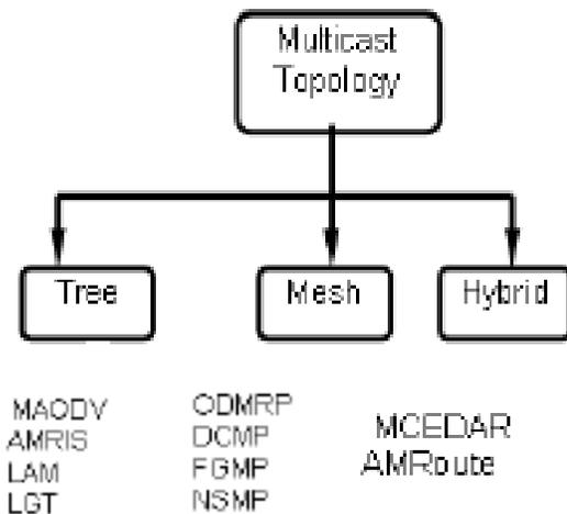
Figure 1: Multicast routing protocols in MANET
