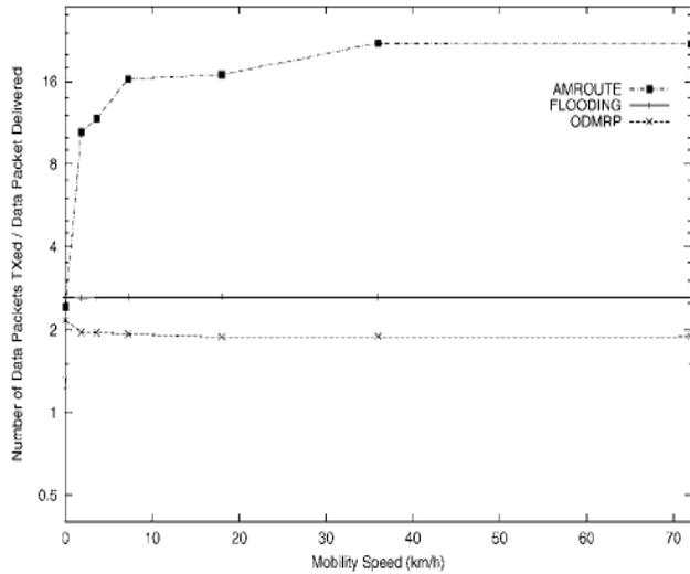
Figure 8: Number of data packets transmitted per data packet delivered as a function of mobility speed.
