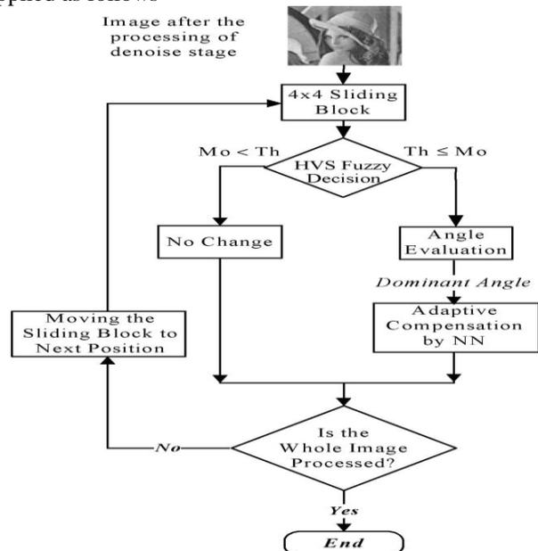
Figure 2: Procedure diagram of the image quality enhancement
