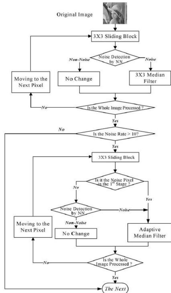
Figure 1: Procedure diagram of the two-level impulse noise removal Impulse Noise Model
