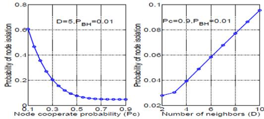
Figure. 2. Effects of Pc and d on node isolation probability.
