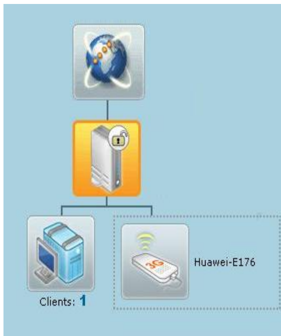
Fig[[]] Router connects with the USB Dongle, Client & World by Internet.
