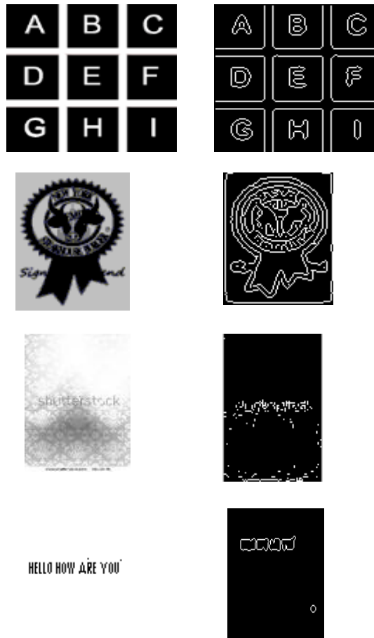
Fig. 11 Results Using Robet Edge Detector ([23]-Original Images)
