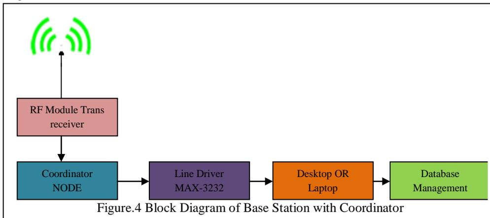
Figure.4 Block Diagram of Base Station with Coordinator
