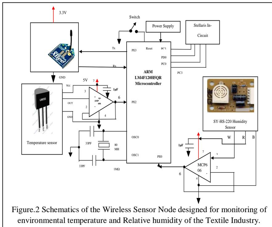
Figure.2 Schematics of the Wireless Sensor Node designed for monitoring of environmental temperature and Relative humidity of the Textile Industry.
