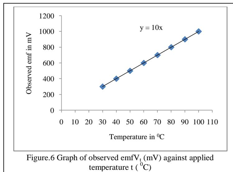
Figure.6 Graph of observed emf  $V_t$  (mV) against applied temperature  $t$  ( $^{\circ}\text{C}$ )
