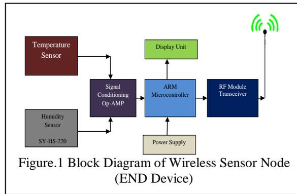
Figure.1 Block Diagram of Wireless Sensor Node (END Device)
