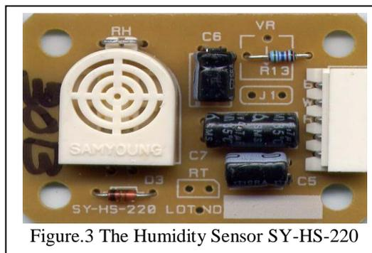
Figure.3 The Humidity Sensor SY-HS-220
