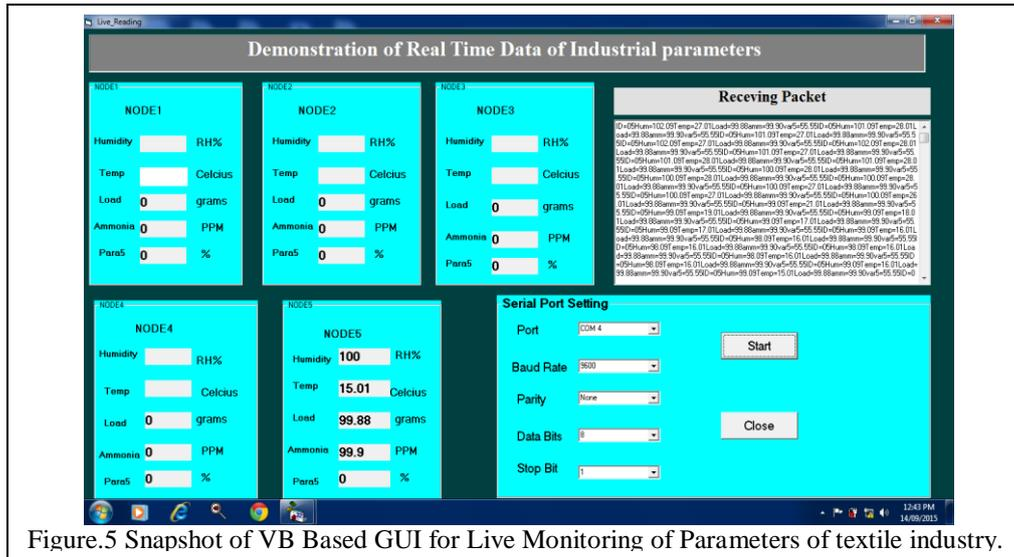
Figure.5 Snapshot of VB Based GUI for Live Monitoring of Parameters of textile industry.
