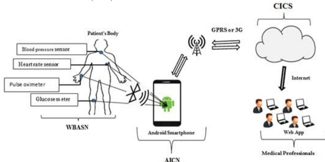
Fig. 1 The BASN-based Mobile Healthcare System Architecture
