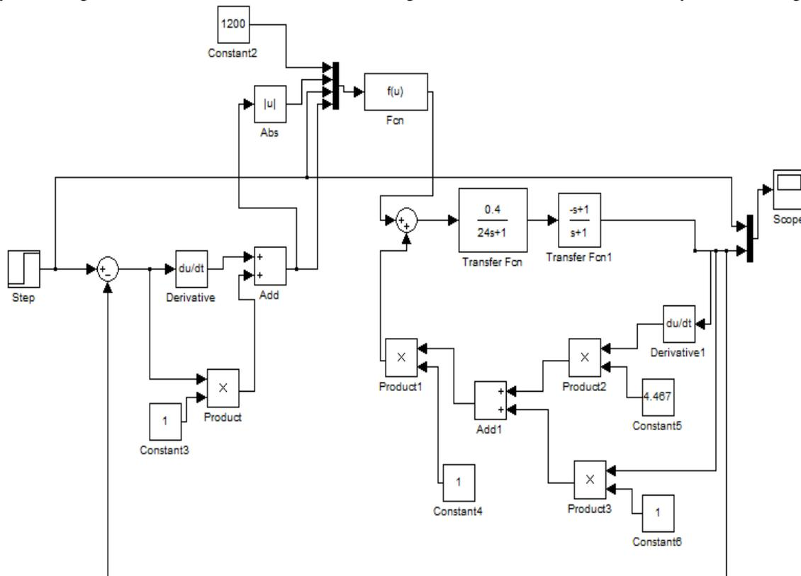
Figure. 5 Block Diagram of Sliding Mode Control
