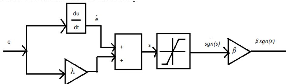
Figure. 4 The block diagram of sliding surface selection
