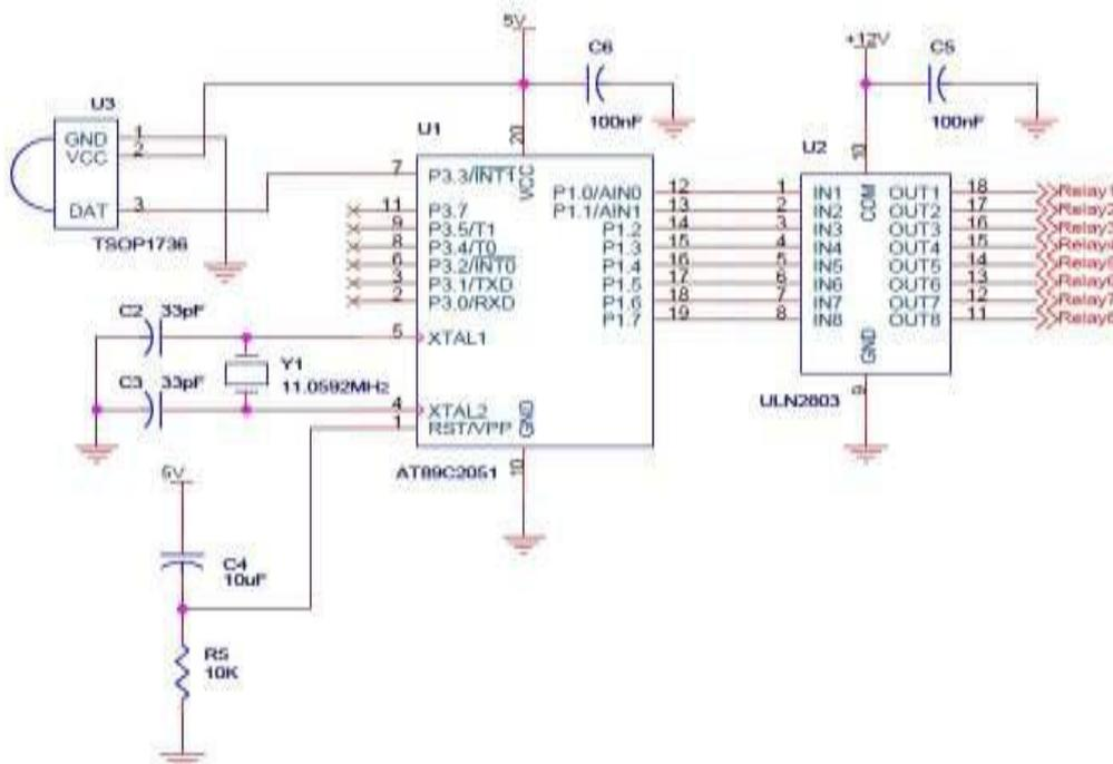
As this paper as mentioned earlier is aimed at controlling 6 home appliances using a TV remote or any remote supporting RC5 Protocol. It controls the on/off process of the appliances interfaced to this circuit. The devices are operated using the keypads 1-8. It performs the function of an IR transmitter which sends pulsed IR rays after modulating the original signal with a carrier of 36 kHz frequency. These signals are received by TSOP 1736 which is our IR receiver.
