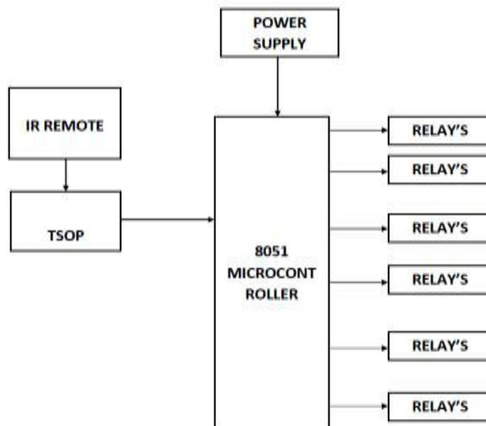
Figure: 1. Block Diagram
