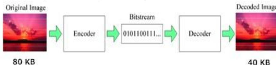
Fig.1. Process of Image Compression
