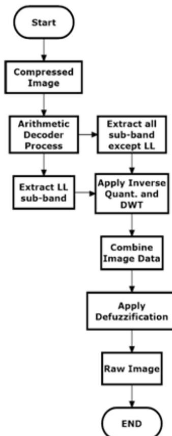
Fig. 5.Decoder of Proposed Methodology
