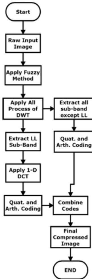
Fig.4. Encoder of Proposed Methodology
