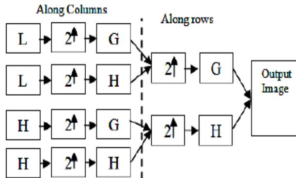
Fig.3 Block Diagram of Reverse DWT
