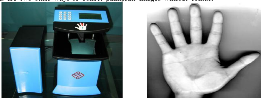
Fig: A CCD-based palmpoint scanner
