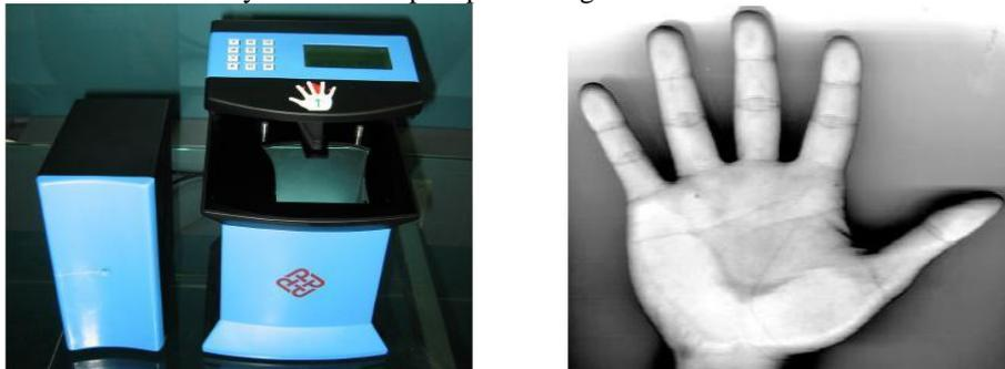
Fig: A CCD-based palmpoint scanner
