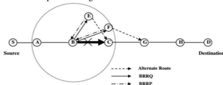
Fig 2. Re-route of data packets in AODV-ABR
