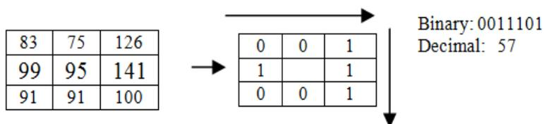
Figure 1 Example of Basic LBP Operator
