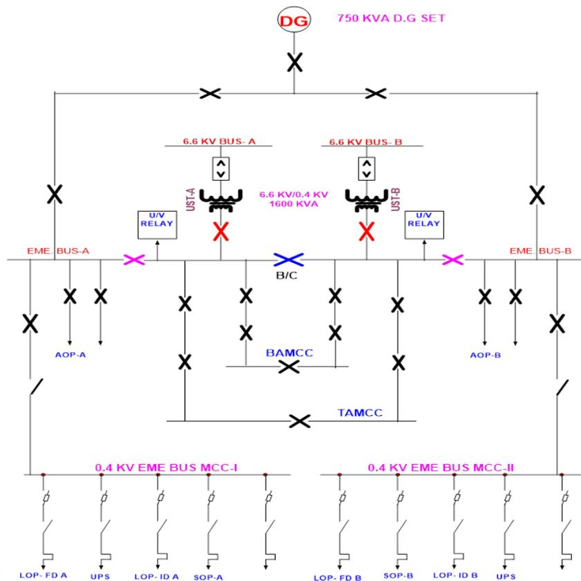
Fig. 4 unit 0.4kv bus and back-up d.g set
