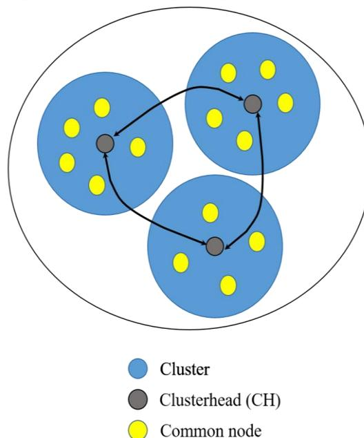
Fig. 1 Clustering Arrangement for a MANET Setup
