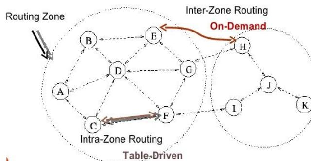
Fig. 5: ZRP routing protocols
