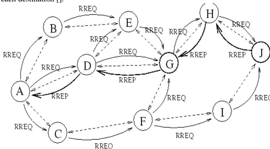
Fig. 2: AODV routing protocols
