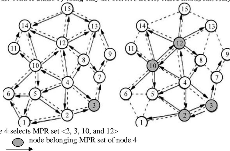
Broadcast packet forward by members of MPR set Flooding the entire network with six transmission using MPR scheme
