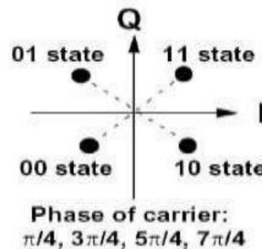
gray code overcome the bit error rate(BER). QPSK represent the four. Due to this its data rate is more than the BPSK. Although maintaining the bandwidth of the signal or data rate of the BPSK but half of the bandwidth required.
