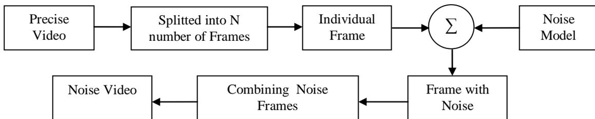
Fig 1: Block Diagram of Noise Model for a Precise Video.
