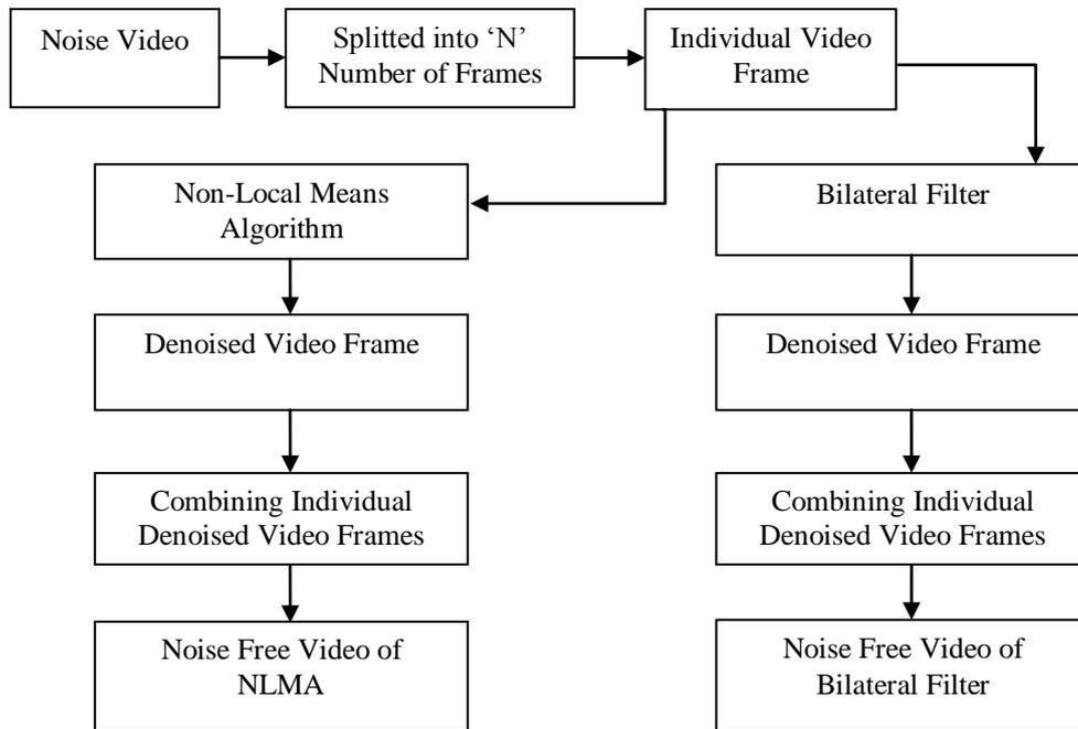
Fig. 3: Block Diagram of 'Video Denoising by Non-Local Means Algorithm and Bilateral Filter'.
