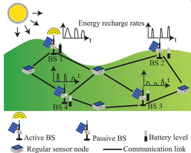
**Fig 1.** A WSN with the proposed scheme that deploys multiple BSs, keeps only one of them active and adaptively re-selects this active BS. At the current time, BS 1 is active. Sometime later, the active BS will be re-selected based on the states of the network, e.g., battery levels. By using this scheme, the temporally and spatially varying energy resources of all BSs are fully utilized.
