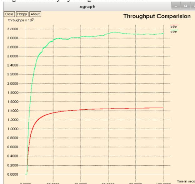
Fig 4: Shows Comparison between base (red) and Proposed (green) values in Throughput.
