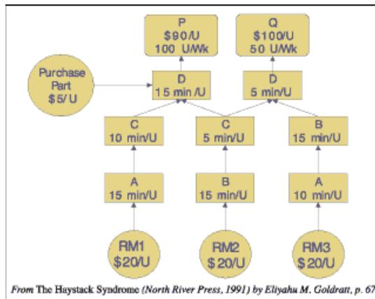
Figure 1: A Simple Process with a Constraint
