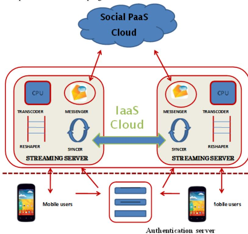
Fig. 1.1: Architecture of cloud dependent portable television buffer streaming
