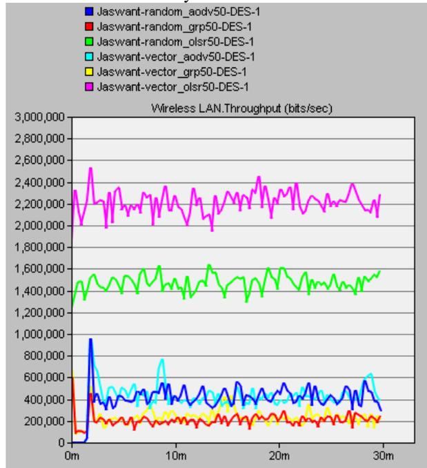
Figure 5. Throughput (bits/sec) comparison in routing protocols with 50 nodes
