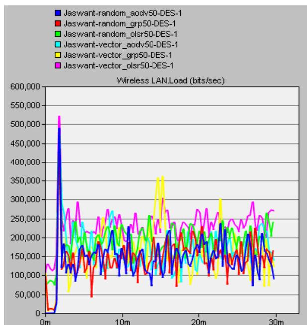
Figure 4. Network Load comparison in three routing protocols with 50 nodes
