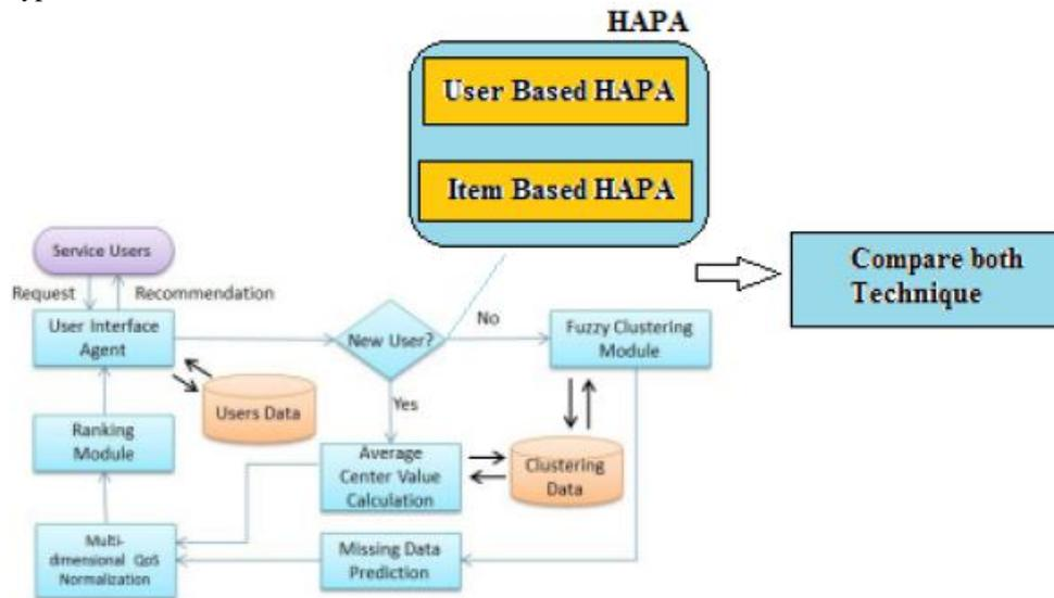
Fig. 1 Architecture of HAPA [8]
