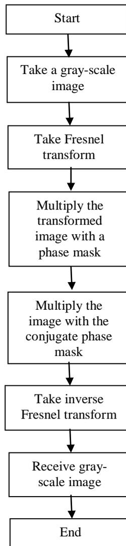
Fig. 2 Flow chart to represent cryptography process using Fresnel transform
