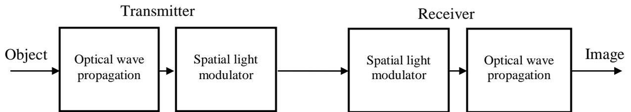
Fig. 1 Optical set-up to implement cryptography process using Fresnel transform
