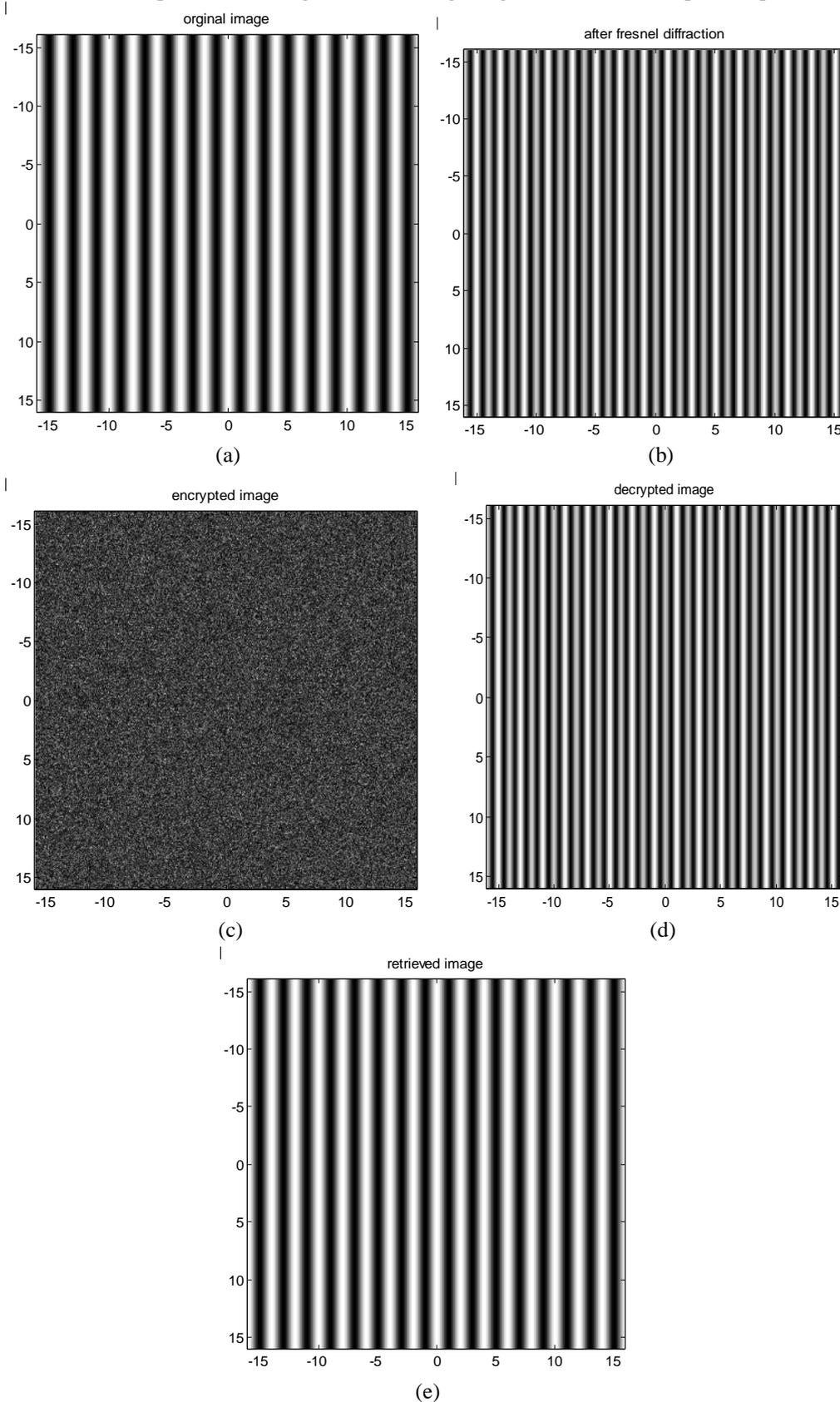
Fig. 3 Outputs at different stages of the cryptography process: (a) image of a sinusoidal grating, (b) Fresnel transform of the sinusoidal grating, (c) output obtained after multiplying the transformed image with a random phase mask, (d) output obtained after multiplying the image in (c) by the conjugate phase mask, (e) final result after taking inverse Fresnel transform.
