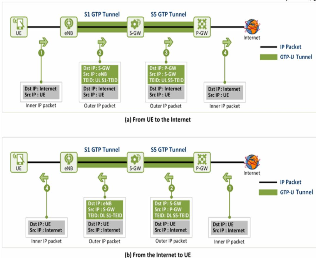
Figure 3. Traffic flow on the LTE network
