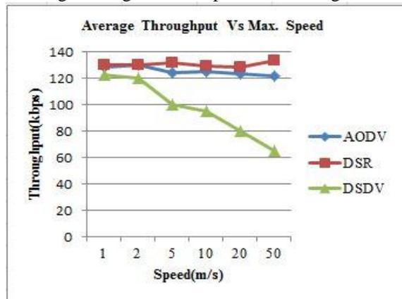
Figure 4: Throughput Vs Speed
