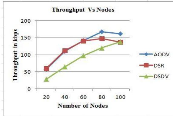
Figure 7: Throughput Vs Numbers of Mobile Nodes
