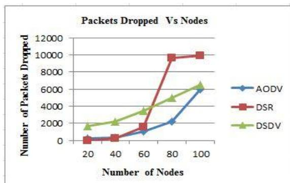
Figure 9: Packets Dropped Vs Number of Mobile Nodes
