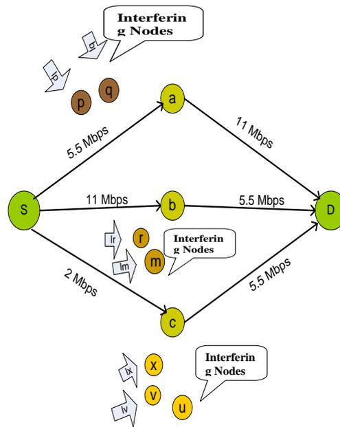
Figure 4.8 Network with interfering nodes with different link rate
