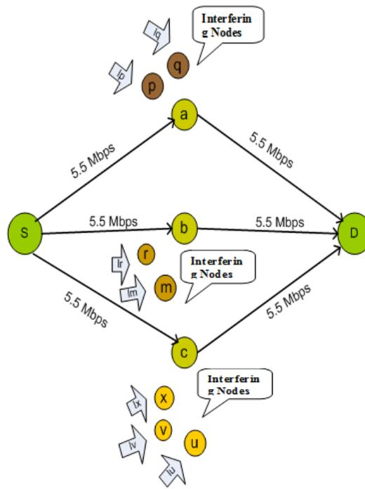
Figure 4.7: Network with interfering nodes for same link rate
