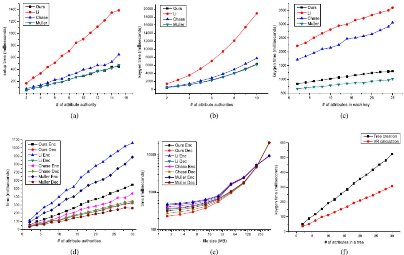
Fig. 2. Experiment result on our implemented prototype system. (a) Setup time. (b) Keygen time with different authorities’ #. 20 attributes per key. (c) Keygen time with different attributes #. 4 authorities. (d) Encryption and decryption time with different attributes number. File size is 100KB. (e) Encryption and decryption time with different file size. 20 attributes in T0. (f) Time to create a privilege tree and decrypt a verification parameter from it.
