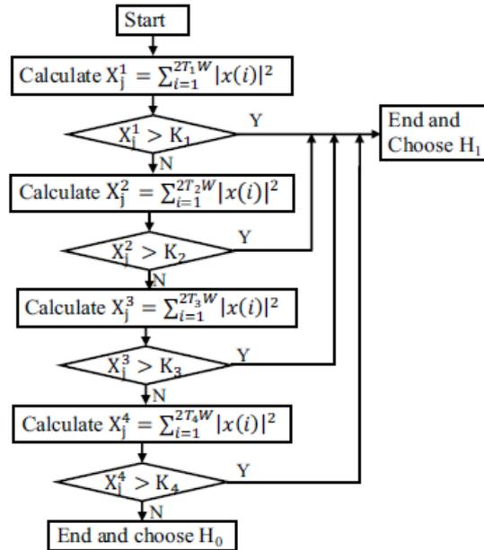
Figure 4 Flow chart of asynchronous energy sensing [7]
