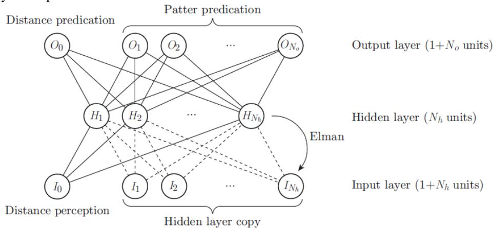
Fig. 4 The architecture of the Elman neural network
