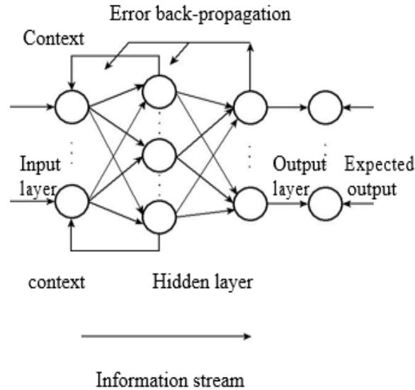
Fig. 2 Internal process analysis of ENN
