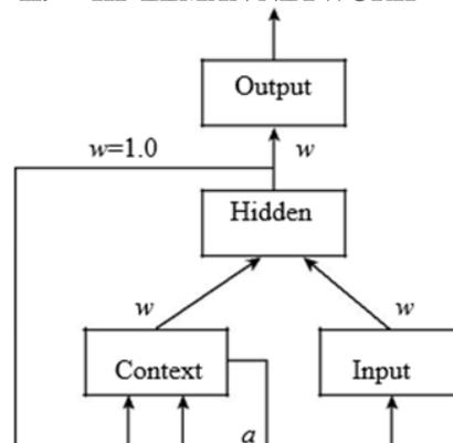
Fig. 1 The structure of the ENN
