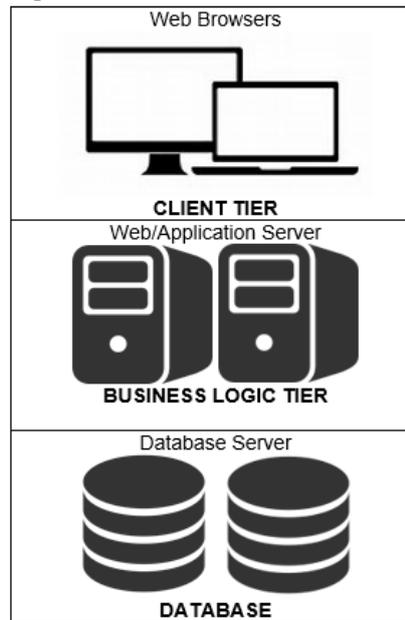
Fig. 3 A 3 Tier Client Server Architecture
