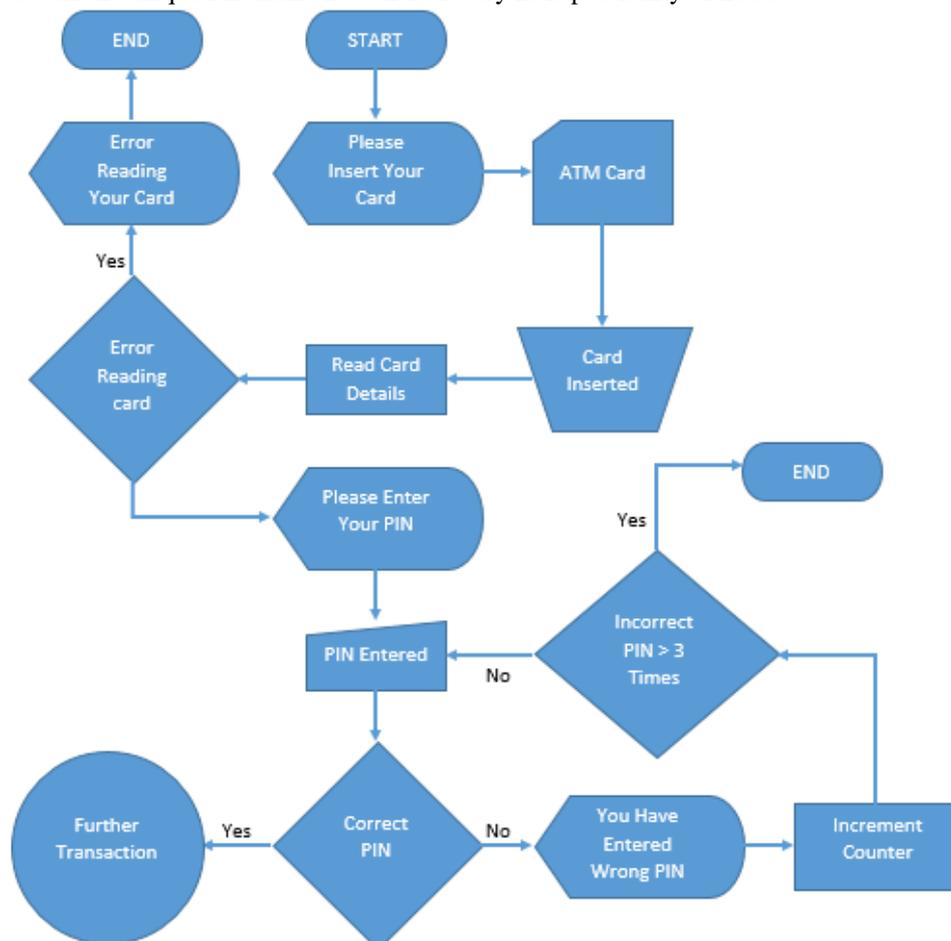
Fig. 4 Flow chart of ATM transaction
