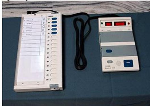
Fig. 1 EVM. Ballot Unit (Left) Control Unit (Right)
