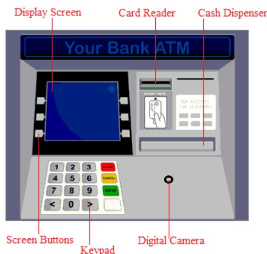
Fig. 2 Automatic Teller Machine (ATM)
