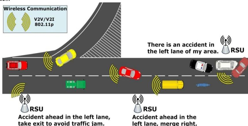
Fig.1. This figure shows the communication scenario among vehicles and road side units using VANET
