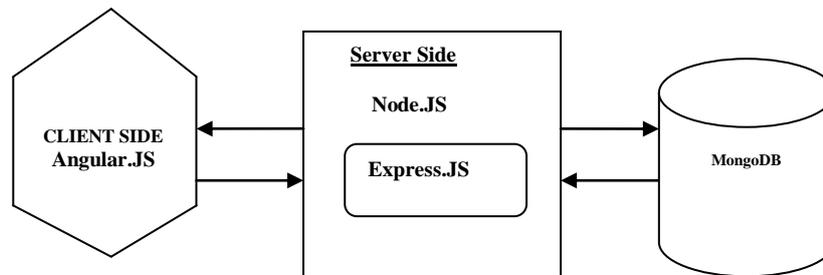
Figure 1: Overview of MEAN stack used in SIMS
