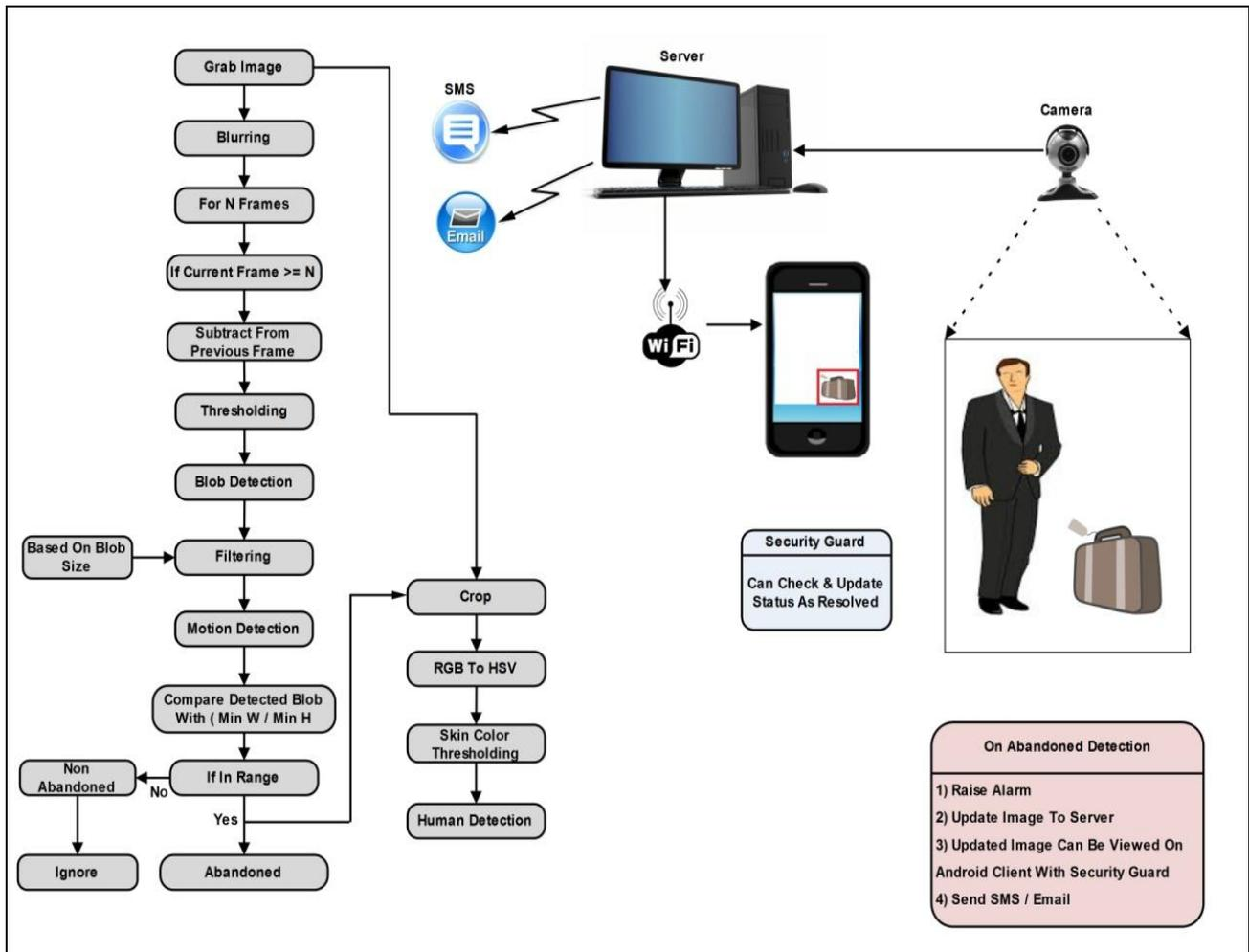
Fig 1: Block Diagram for proposed system
