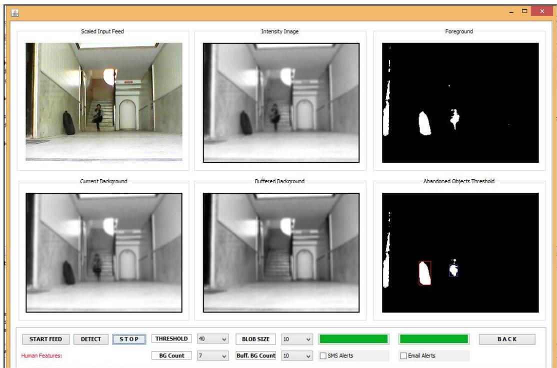
Fig 6: Abandoned Object Detection in the Presence of Human
