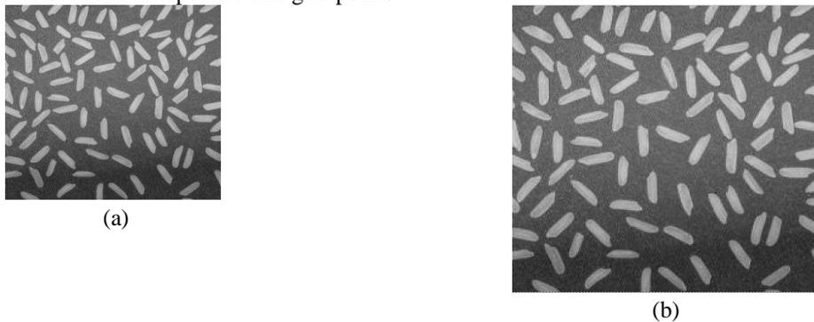
Fig.4 Image (a) is the original image and (b) is zoomed image using bicubic interpolation
