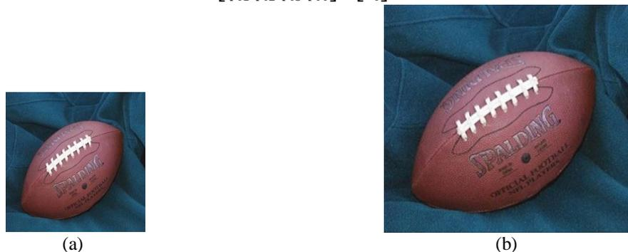
Fig. 1 Image formed by using Bi-Cubic Interpolation (a) Original Image (b) Zoomed Image
