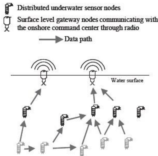
Fig. 1. An representation of the portable UWSN design for long-term non-time-basic amphibian checking applications. Submerged sensor framework is a exceptionally new research area. Recent articles furthermore give great surveys on this area.
