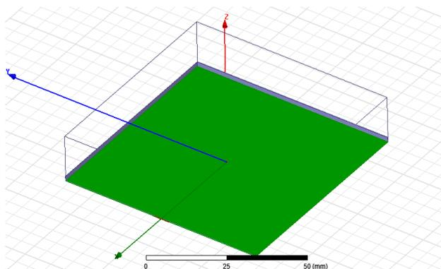
Fig. 4.9. Bottom View of a Rectangular Microstrip Patch Antenna for a Microstrip Line feed Technique
