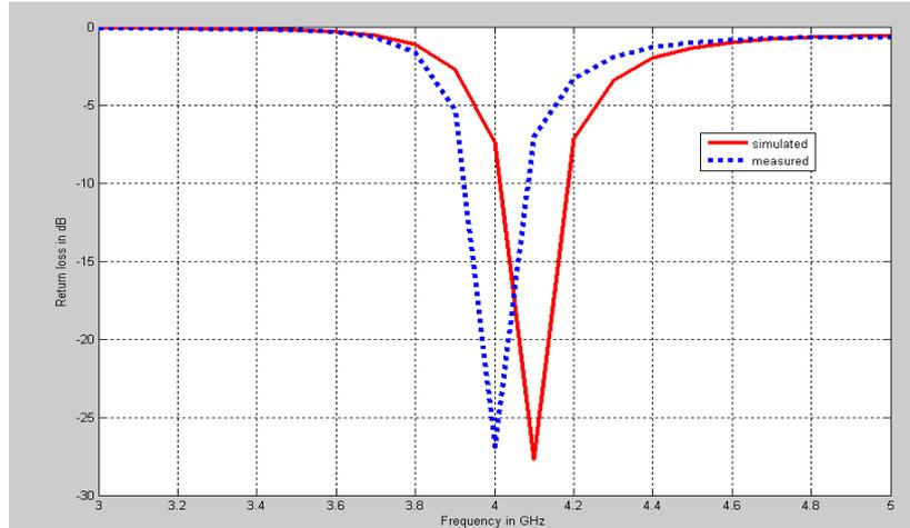
Fig. 5.4. Comparison between Simulated and Measured Return Loss of a Rectangular Microstrip Patch Antenna for a Co-axial Probe feed Technique
