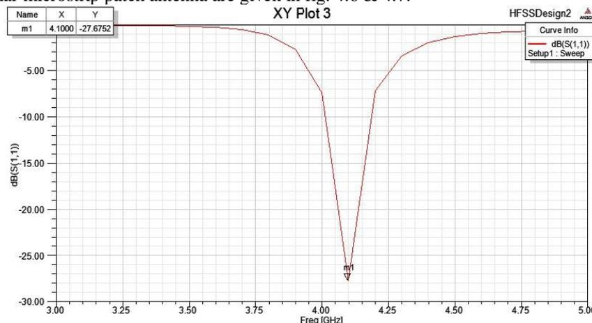
Fig. 4.3. Simulated Return Loss of a Rectangular Microstrip Patch Antenna for a Co-axial Probe feed Technique
