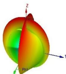
Fig. 4.12. Simulated Directivity of a Rectangular Microstrip Patch Antenna for a Microstrip Line feed Technique
