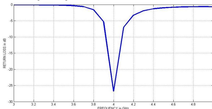
Fig. 5.3. Measured Return Loss of a Rectangular Microstrip Patch Antenna for a Co-axial Probe feed Technique
