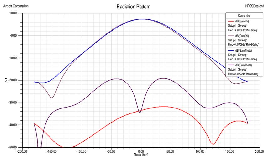
Fig. 4.11. Simulated Gain Plot of a Rectangular Microstrip Patch Antenna for a Microstrip Line feed Technique
