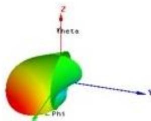
Fig. 4.7. Simulated RHCP of a Rectangular Microstrip Patch Antenna for a Co-axial Probe feed Technique
