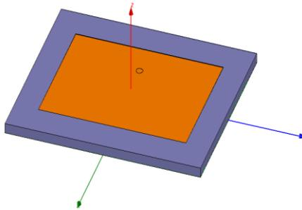
Fig. 4.1. Top View of a Rectangular Microstrip Patch Antenna for a Co-axial Probe feed Technique
