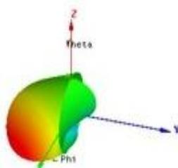
Fig. 4.14. Simulated RHCP of a Rectangular Microstrip Patch Antenna for a Microstrip Line feed Technique
