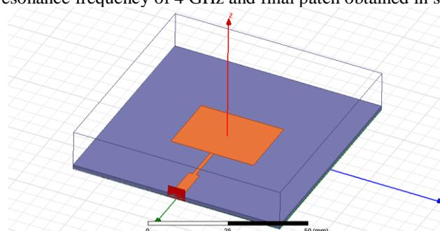
Fig. 4.8. Top View of a Rectangular Microstrip Patch Antenna for a Microstrip Line feed Technique
