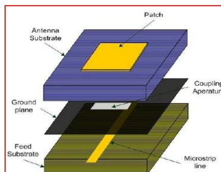
Fig. 2.3. A model of Aperture Coupled Feed
