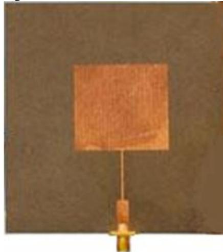
Fig. 5.5. Fabricated View of a Rectangular Microstrip Patch Antenna for Microstrip Line feed Technique
