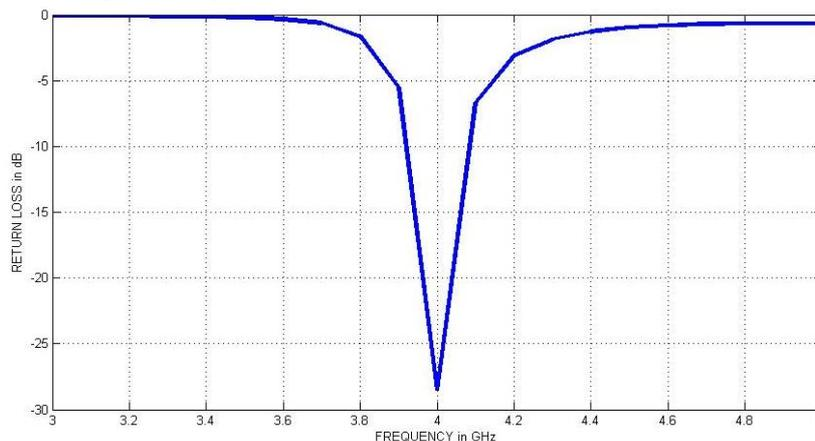
Fig. 5.6. Measured Return Loss of a Rectangular Microstrip Patch Antenna for a Microstrip Line feed Technique
