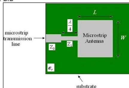
Fig. 2.2. A model of Microstrip Feed
