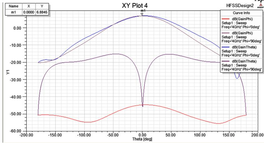
Fig. 4.4. Simulated Gain Plot of a Rectangular Microstrip Patch Antenna for a Co-axial Probe feed Technique
