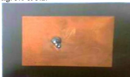
Fig. 5.1. Fabricated Top View of a Rectangular Microstrip Patch Antenna for a Co-axial Probe feed Technique
