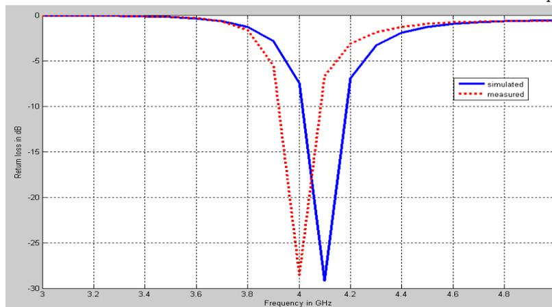
Fig. 5.7. Comparison between Simulated and Measured Return Loss of a Rectangular Microstrip Patch Antenna for a Microstrip Line feed Technique
