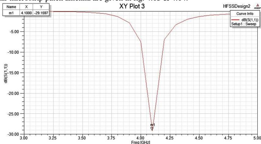
Fig. 4.10. Simulated Return Loss of a Rectangular Microstrip Patch Antenna for a Microstrip Line feed Technique
