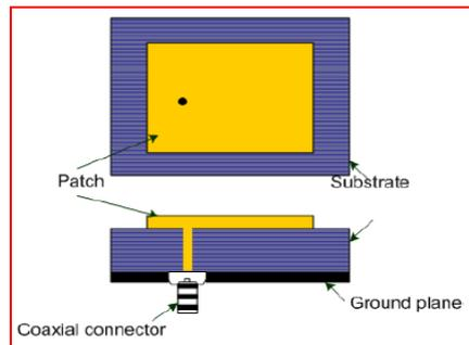
Fig. 2.1. A Model of Co-axial Feed
