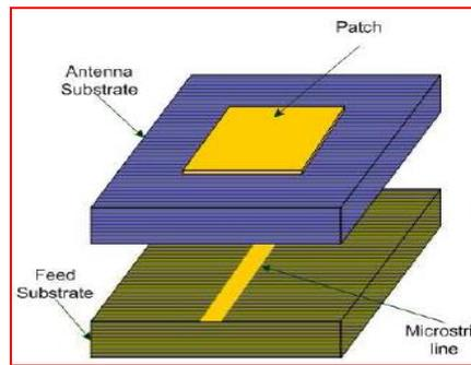
Fig. 2.4. A model of Proximity Coupled Feed
