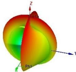
Fig. 4.5. Simulated Directivity of a Rectangular Microstrip Patch Antenna for a Co-axial Probe feed Technique
