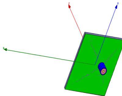
Fig. 4.2. Bottom View of a Rectangular Microstrip Patch Antenna for a Co-axial Probe feed Technique
