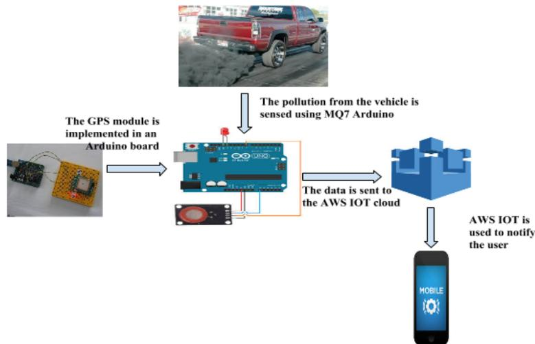
Fig 3.1 An Architecture of Smart Pollution Detection system
