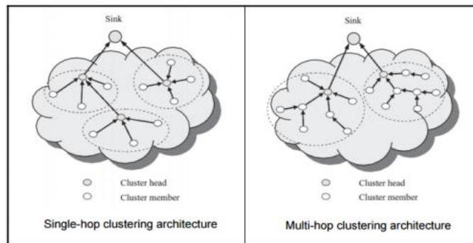
Fig. 3. Hierarchical Architecture of WSN[13]
