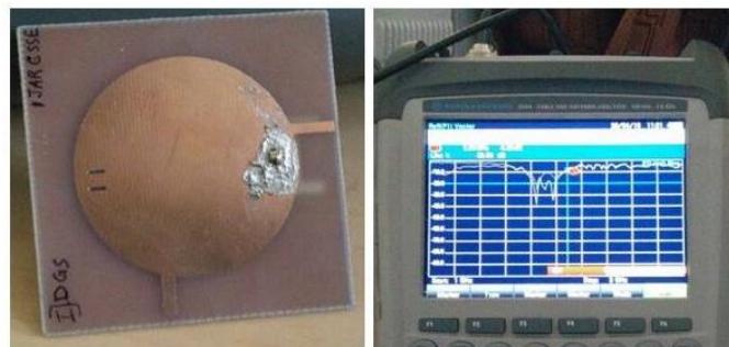
Fig 12 : The hardware of the proposed antenna and Simulation reading of the hardware using R&S Antenna analyser
