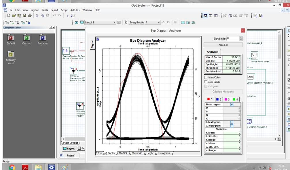
Fig: Showing the results for the eye diagram and Q factor for input and output peak power.
