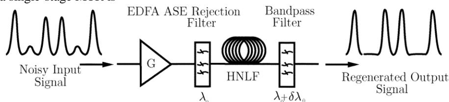
It employs a high-power erbium-doped fiber amplifier (EDFA) to boost the peak power of the incoming noisy signal to the power level that is high enough to cause spectral broadening through the SPM. The amplified signal is first passed through an ASE rejection filter that rejects the out-of-band ASE noise added by the high-power EDFA. The ASE filter is
