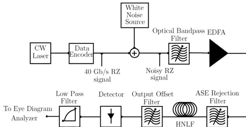
Fig. 2. Setup used for simulating numerically the operation of an MTR.
