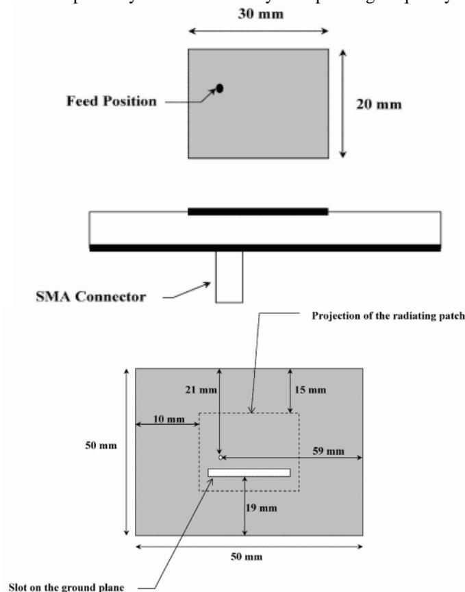
Figure 1: Layout of the antenna with single rectangular slot in the ground plane
