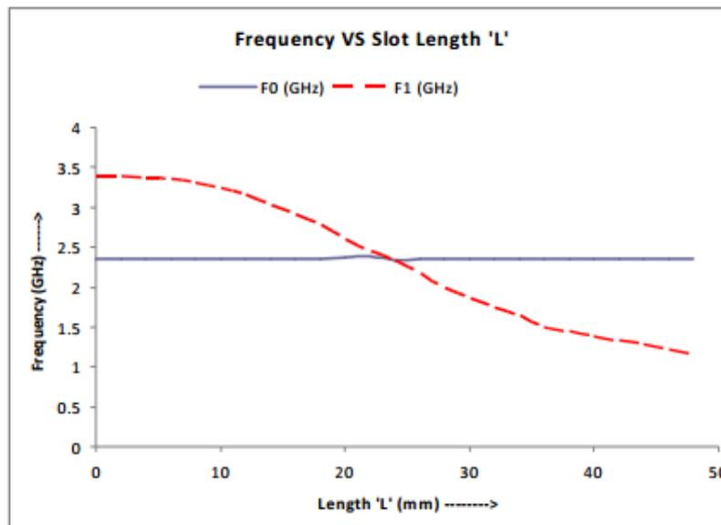
Figure 3: Variation of the two resonant frequencies with slot length “L”
