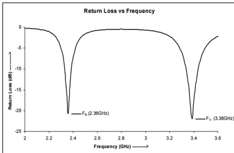
Figure 2: Simulated return loss of the antenna with slot length “L”= 0 mm
