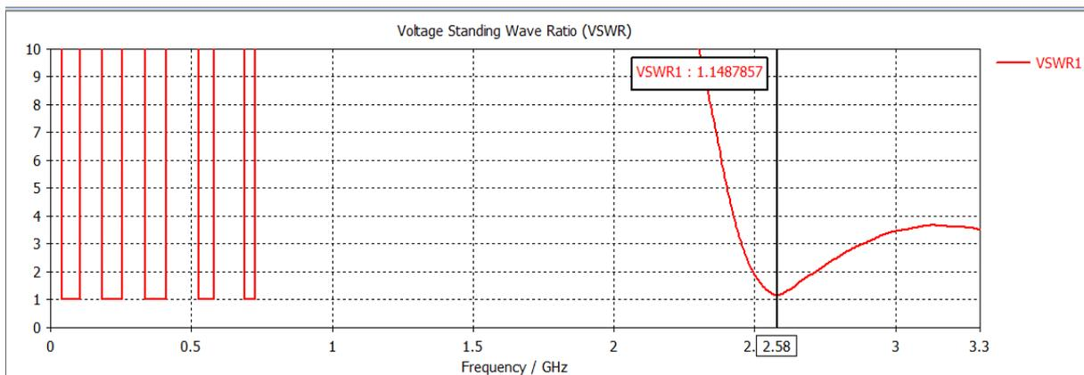
Fig. 7 VSWR plot the proposed antenna at 2.58 GHz
