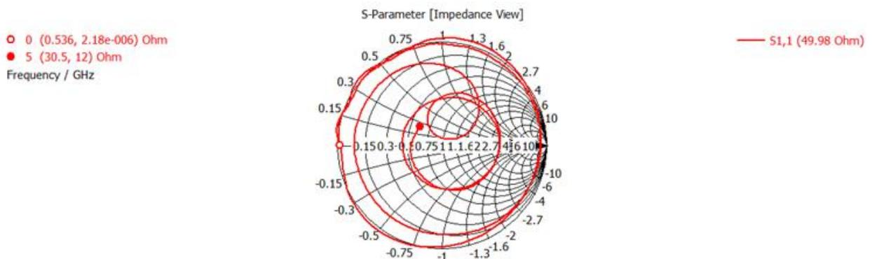
Fig. 8 Smith chart plot of the proposed antenna at 2.58 GHz
