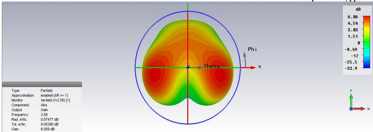
Fig. 5 Gain of the proposed antenna at 2.58 GHz
