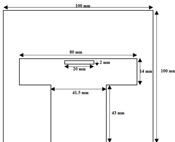
Fig. 3 Top view of the proposed antenna
