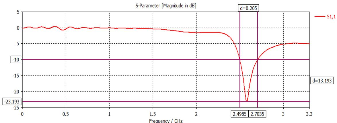
Fig. 4 Return loss plot of the proposed antenna at 2.58 GHz
