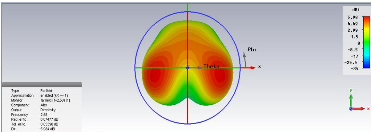
Fig. 6 Directivity of the proposed antenna at 2.58 GHz
