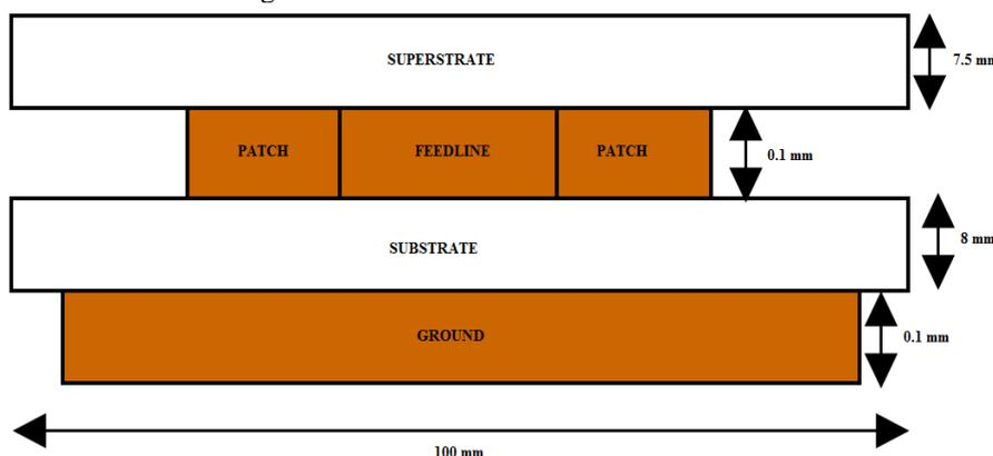
Fig. 1 Front view of the proposed antenna
