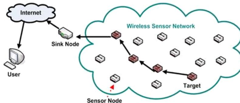
Fig.1. Example of a wireless sensor network
