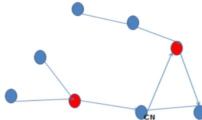
Fig.2 Scenario of multi node failure as failure of two nodes(red nodes) introduces a conflict for node CN since in many single node failure recovery schemes it has to be engaged in the recovery process for both of them
