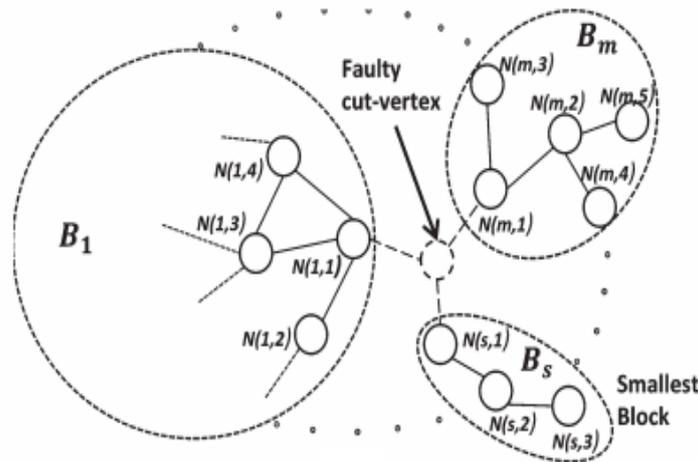
Fig.6 (a) WSAN before a cut vertex fails
